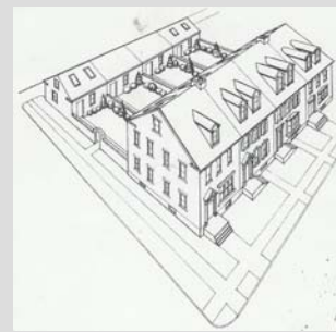
Townhouses with garages accessed from a laneway. This type of development creates a walkable street frontage.
