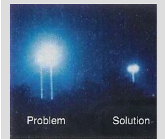
Fully shielded fixtures, such as the “light-structure green™” stadium fixtures shown on the right, minimize light spillage on adjacent properties. Since they are more energy efficient, they are also less expensive to operate.
